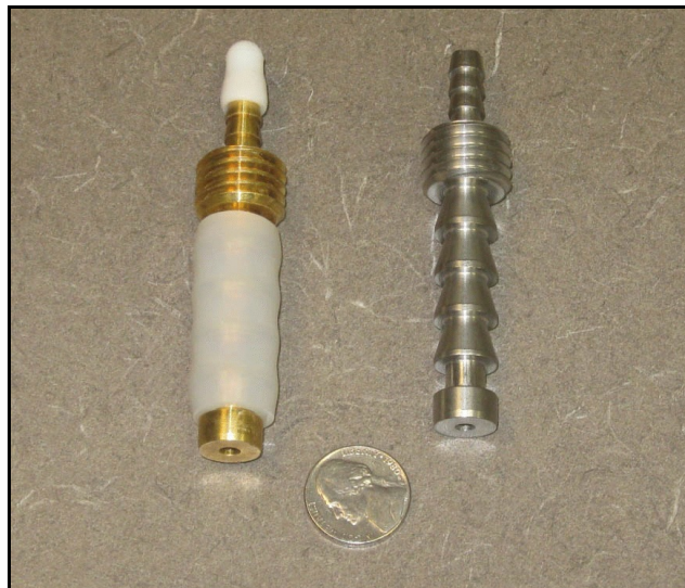
Figure 1. Vapor Pin™ Sub-Slab Samplers.
