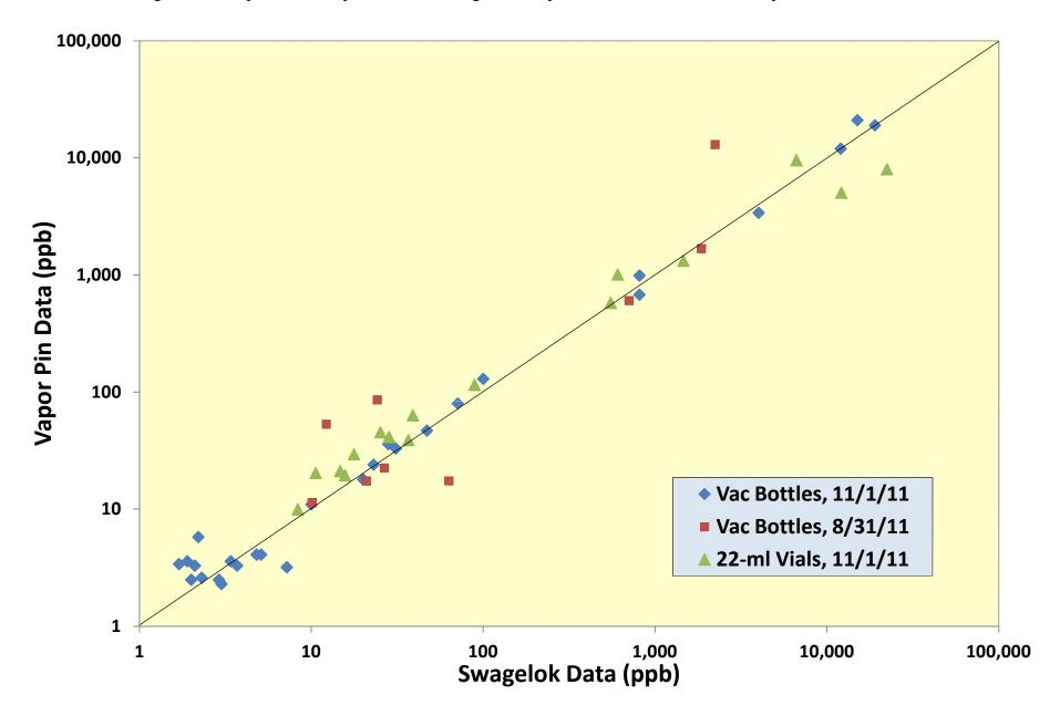
Figure 2. Comparison of Vapor Pins<sup>TM</sup> to Swagelok Sample Points, with Data from Sample Point 12 Removed.
