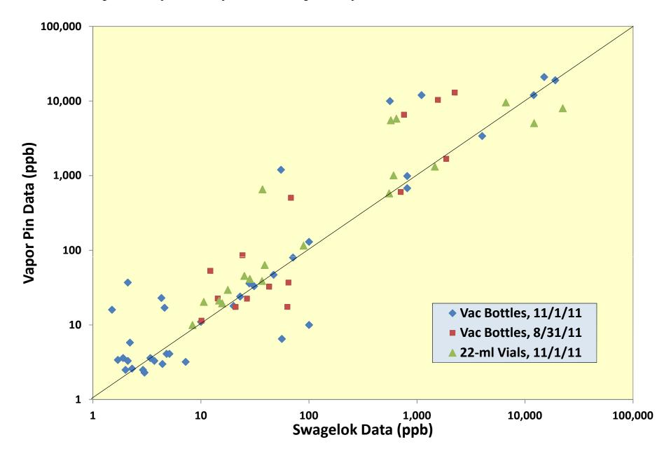
Figure 1. Comparison of Vapor Pins<sup>TM</sup> to Swagelok Sample Points.
