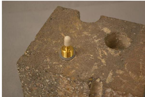
Figure 3. Vapor Pin installé
