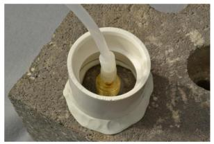
Figure 3. Water dam used for leak detection
