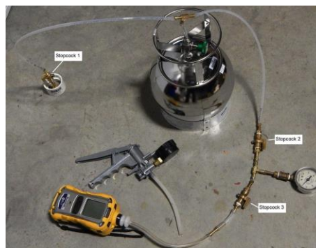
Figure 1. Example of Sub-Slab Sampling and Leak-Test Setup
