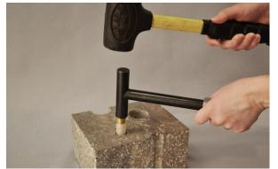
Figure 2. Installing the VAPOR PIN®
