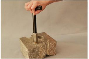
Figure 7. Removing the VAPOR PIN<sup>®</sup> sampling device
