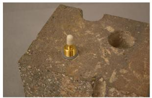
Figure 3. Installed VAPOR PIN<sup>®</sup> sampling device
